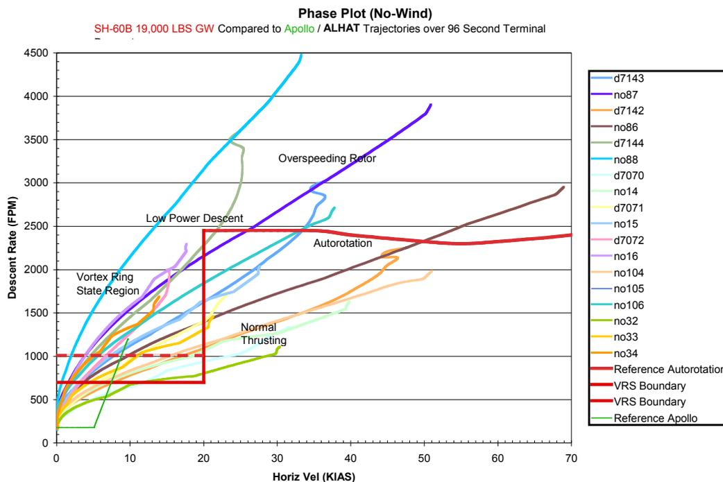
**Figure 13** ALHAT Trajectories Compared to Helicopter Descent Capabilities
