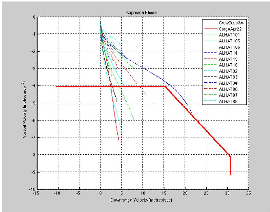
**Figure 15** LDAC and ALHAT Approach Trajectories and Vortex Ring State Region
